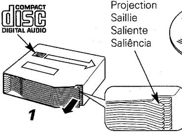
**1.** Make sure the disc magazine is the right way up with the "disc" logo on the top. Pull the tray out by the projection.
