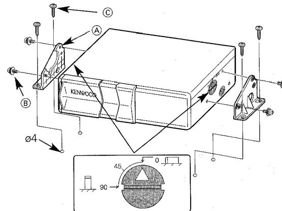
**■ Vertical installation / Installation verticale / Instalación vertical / Instalação vertical**
